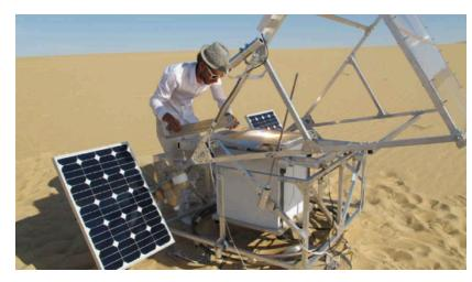
Glass is printed in the Sahara desert with sand "ink" and a solar powered 3D printer.
